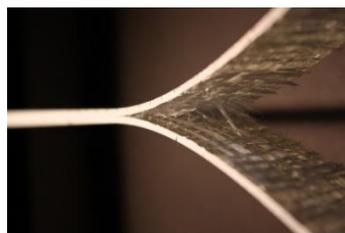
Fig.2: Mode I crack opening
